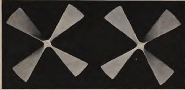
Fig. 37a. —Right and left-hand four-blade screws used in my experiments for ascertaining the comparative efficiency between screws placed in front and in the rear of the machine.
